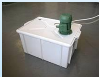
Coolant re-circulating system with pump and sump assembly, Included in the C series machines
