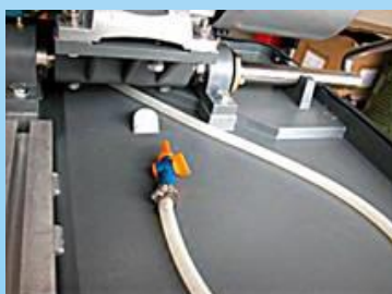
Flushing hose to keep the working top clean from residues.
