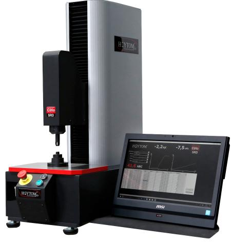
This model has been developed to perform tests using the Rockwell scale (with loads of 60, 100 and 150 kp), and the Rockwell superficial scale (loads of 15, 30 and 45 kp), but can also apply additional loads for other tests, such as Brinell or Vickers. It is comprised of a motorised frame, which includes the load application systems (which employ a computer controlled force transducer).
